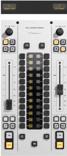
The Call Controller module has two faders plus integrated line switching controls with Status Symbols, for on-console control of advanced Telos broadcast phone systems. Available in standard and motorized-fader versions.
