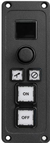
In-studio accessory panel mounts in tabletop or turret. Provides remote control of mic on/off functions; dedicated Mute and Talkback buttons give talent full control of their position. Volume/selection knob allows users to select their headphone monitor source; display readout confirms their choice. Connects to Fusion Interface Board CANbus using CAT-5 cable. 6" x 2", requires 2" mounting depth.
