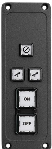
Special accessory panel for producers source profiles, which mounts in tabletop or turret to provide remote control of mic on/off functions. Includes dedicated Mute key. Two Talkback keys allow producers to talk to control room board op, studio guests, or codecs. Requires one free Axia GPIO port per panel. 6"x 2", requires 2" mounting depth.
