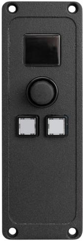
In-studio accessory panel with volume/selection knob mounts in tabletop or turret to allow users to select their headphone monitor source; display readout confirms their choice. Two preset buttons let talent quickly recall frequently-listened-to sources. Connects to Fusion Interface Board CANbus using CAT-5 cable. 6"x 2", requires 2" mounting depth.
