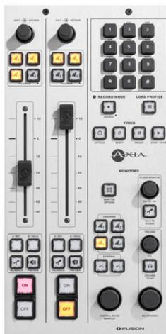
For studios where expert monitor controls are not needed, the Standard Monitor/Navigation module is a space-saving design that incorporates two faders in addition to the numeric entry/dial pad and basic Monitor/Headphone controls.
