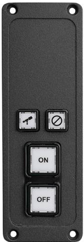
In-studio accessory panel for remote control of mic on/off functions. Mounts in tabletop or turret; includes dedicated Mute and Talkback buttons. Requires one free Axia GPIO port per panel. 6"x 2", requires 2" mounting depth.
