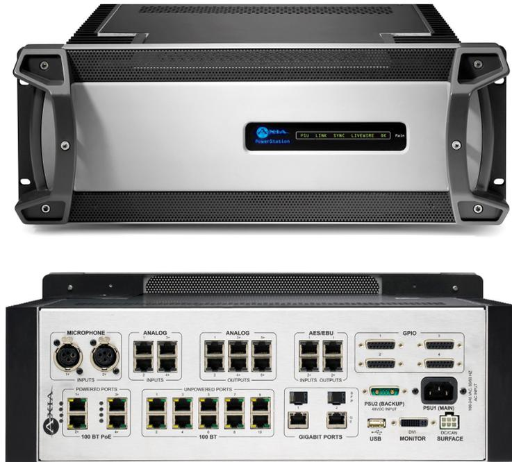
PowerStation is an “integrated console engine”, an all-in-one devices that makes it very easy to install Axia studios and Fusion consoles. Inside that ruggedly handsome case you’ll find a super-powered DSP mixing engine, husky power supply sourced from telecom gear designed for harsh environments, plenty of built-in digital, analog and mic I/O, plus EQ, voice processing — and even a custom, built-for-broadcast Ethernet switch with Gigabit connectivity.
